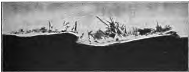
FIG. 64.—Needle-like crystals of prismatic sulfur.
